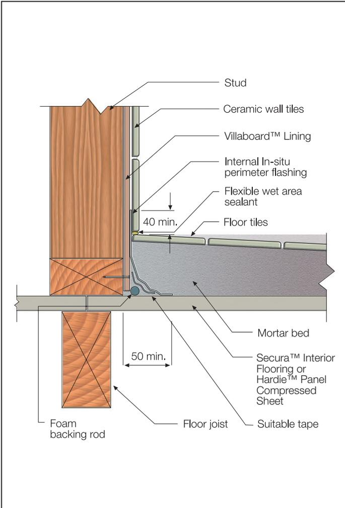
**FIGURE 7 INTERNAL FLASHING**
