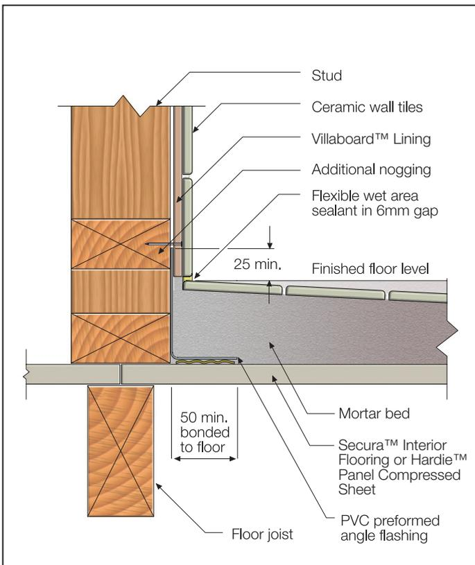
**FIGURE 6 EXTERNAL PERIMETER FLASHING - VILLABOARD™ LININGS FINISHED WITH TILES**
