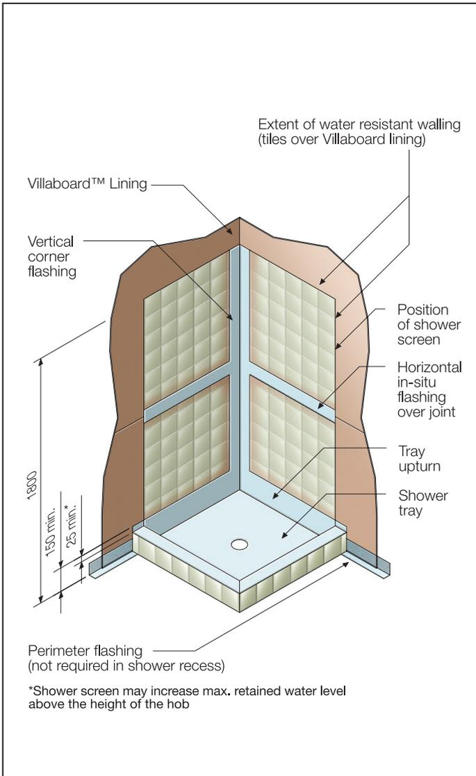
FIGURE 11 INTERNAL MEMBRANE
