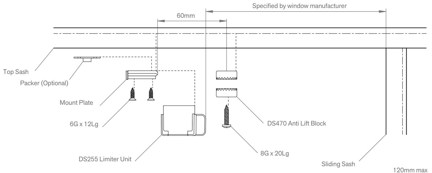
**1.** Use the *mount plate* to mark two centre holes at the distance specified by the window manufacturer from the sliding sash.
