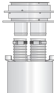
As in step 1, unscrew the flue clamps until they fit over each of the flue pipes. Slide the two flues over the corresponding pipes on the base of the cowl.
