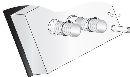
Stretch out the end of each flexible flue pipe. Slide the two flexi flue pipes over the corresponding pipes at the rear of the firebox.
