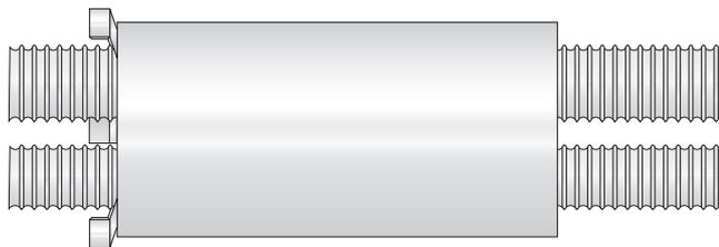
Feed two flexi flues through the 900mm stainless steel flue pipe.
