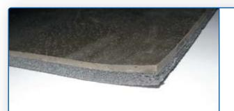
When applied to floors the foam side should face DOWN onto timber boards or concrete. Joins should butt tightly and can be held in place by clouts or InsulTape until flooring is laid. The foam side joins can be spot glued to concrete floors with moisture cured one part polyurethane glue.
