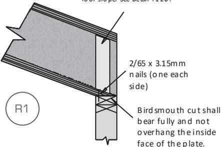
Web stiffeners required each side of SmartJoist. Bevel cut stiffeners to match roof of slope. See Detail F13.
