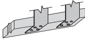
While double joists shown in the above diagram, it is only necessary when loads exceed the capacities of single joist cantilevers.
