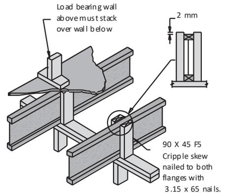
NOTE: Detail F7 with blocking panel is required for bracing walls.
