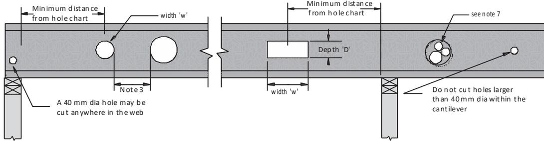
Note: The most accurate method to design the allowable web penetration size and distance from support for SmartJoists is to use the SmartFrame software. The table below will give conservative results in some instances. Also, advice on hole size and location may be obtained by contacting the Technical Support Helpline on 1300 668 690 or at [techsupport@tilling.com.au](mailto:techsupport@tilling.com.au).
