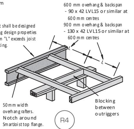
Note: Tiedown details to be designed to AS 1684.2 for the respective wind loads with the SmartFrame software
