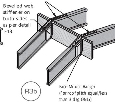
Joist shall be designed using design properties when "L" exceeds joist spacing.
