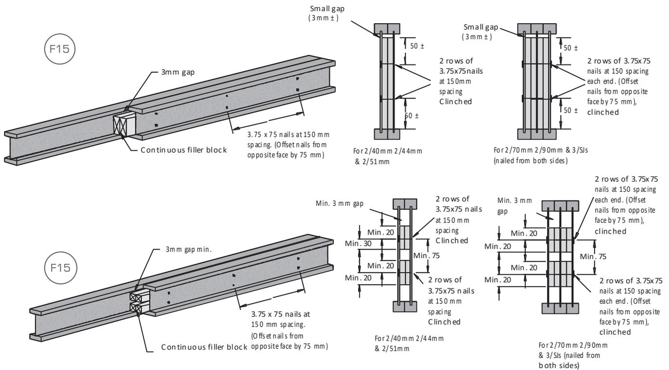
**(b) SmartJoist MultiJoist Clips MJC**
