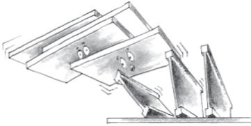
DO NOT ALLOW WORKERS OR LOADS ON SmartJoists UNTIL ALL BLOCKING, HANGERS, RIM JOISTS, NAILING AND TEMPORARY BRACING ARE INSTALLED AS SPECIFIED BELOW. SERIOUS ACCIDENTS OR INJURY CAN RESULT FROM FAILURE TO FOLLOW THESE GUIDELINES.
