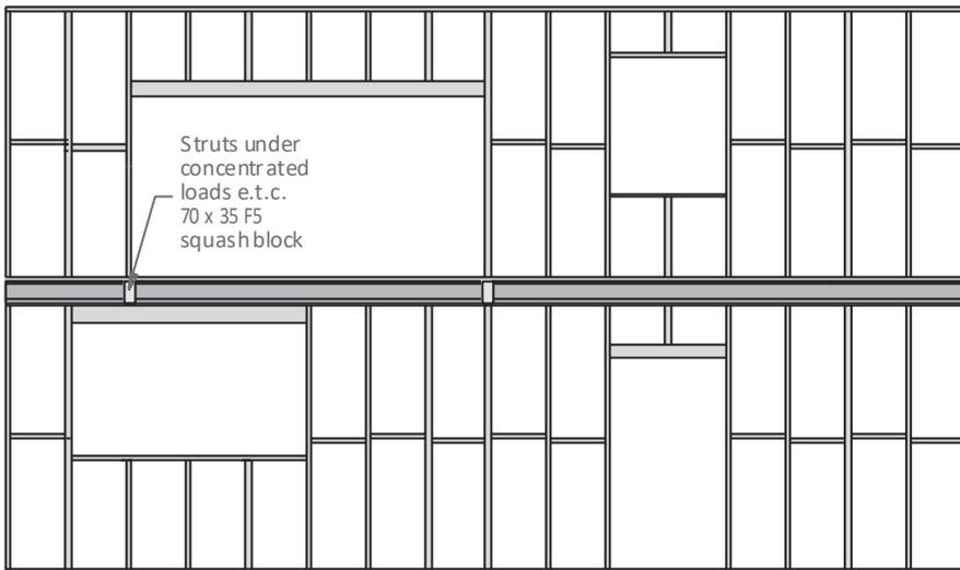
Fix 90x45mm F5 compression block to SmartJoist where load exceeds 6.5 kN\*
