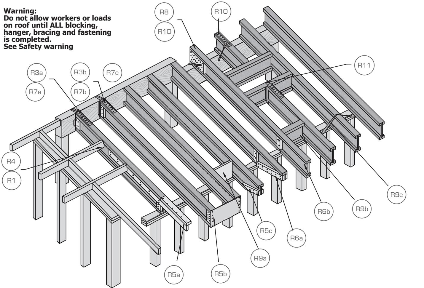
Web stiffeners required each side of SmartJoist. Bevel cut stiffeners to match roof of slope. See Detail F12b.
