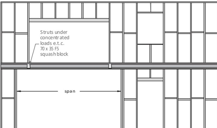
Single (and double) SmartJoists are adequate to transfer uniformly distributed compression loads up to 29 kN/m per joist from loadbearing walls to a continuous rigid support below.
