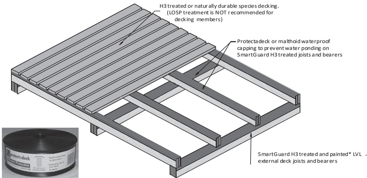
Recommended proprietary top protection for joists and bearers
