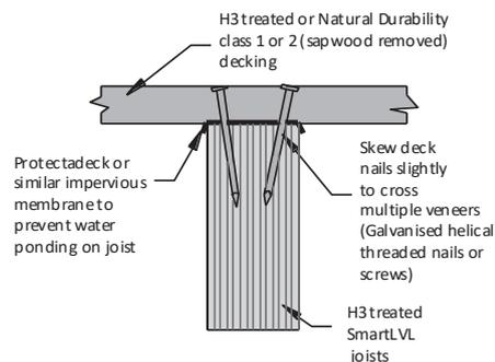
Recommended Fastening to SmartLVL Deck Joists.
