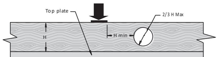
5. For multiple holes, the clear spacing between holes shall be at least two times the diameter of the larger hole, or twice the length of the longest rectangular hole. This minimum hole spacing does not apply to holes of 40 mm or less in diameter, which can be placed anywhere in the rim board (see note 1 for holes over opening) except that the clear distance to the adjacent hole shall be 75 mm minimum.
