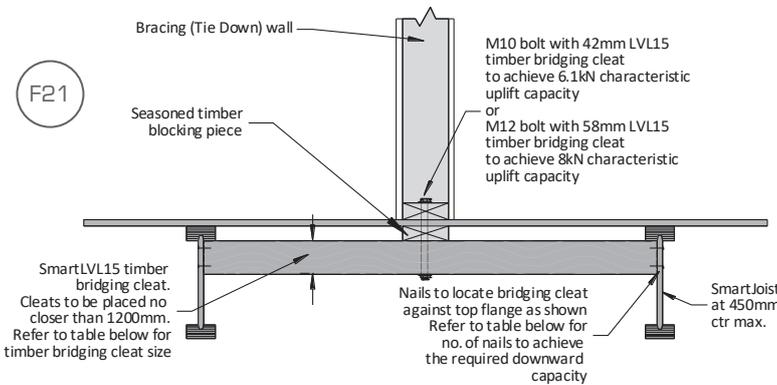
**DO NOT DRILL THROUGH EITHER FLANGE OF SmartJoists unless they are fully supported on wall plate or similar**
