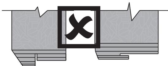
**DO NOT OVER CUT FLANGES. SUBSTANTIAL REDUCTIONS IN CAPACITY MAY OCCUR IF FLANGES ARE OVER CUT**
