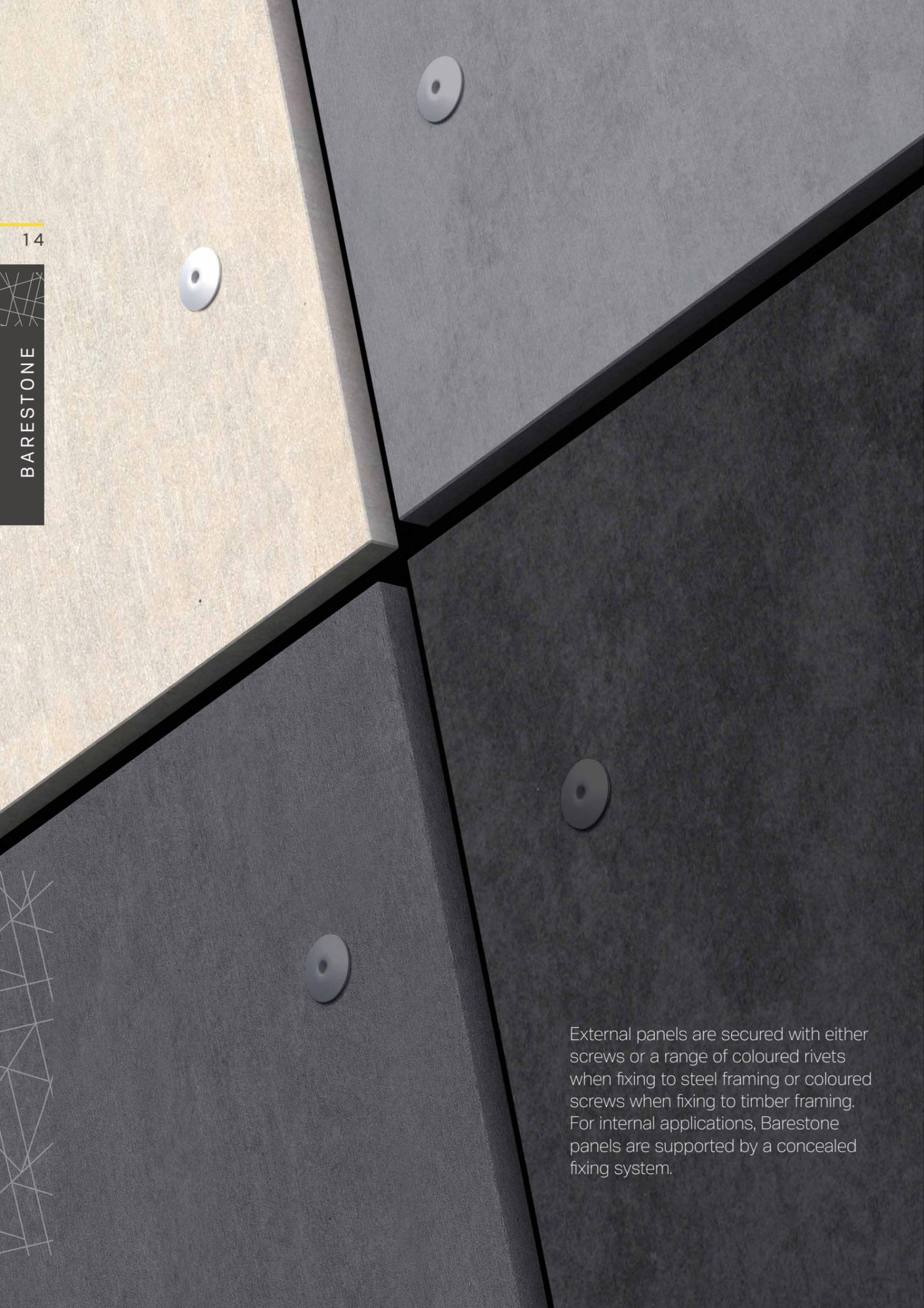
External panels are secured with either screws or a range of coloured rivets when fixing to steel framing or coloured screws when fixing to timber framing. For internal applications, Barestone panels are supported by a concealed fixing system.
