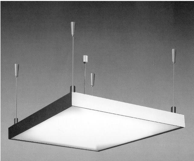
**High Output LED** Pendant light panel. the main body is manufactured from die cast aluminium with ultra pure aluminium. Supplied as standard with opal diffuser panel. The LED driver is remote mounted in the ceiling cavity. Using new generation Led the pendant has 430 x 0.2w LEDs. Supplied in silver powder coated paint finish. Suspension length 1metre
