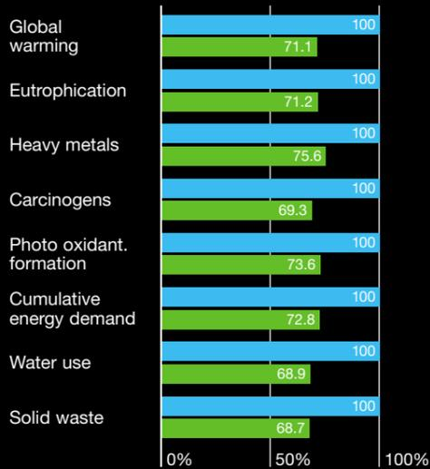
Comparing 1 kg material ‘Pure cement’ with 1 kg material ‘30% Slag’; Method: SimaPro 3.0 Eco-indi Australian Database/Australia revised/characterisation
