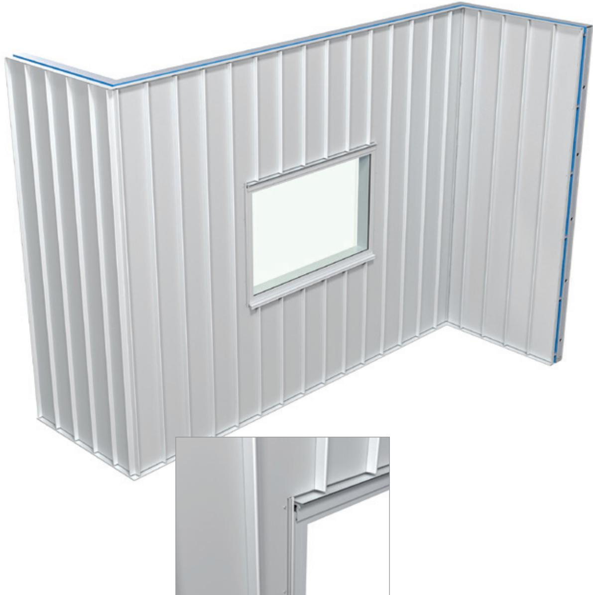
Install packers adjacent to TRM0201b and trim the raised hook/starter section from the length of the Seam panel. Install this trimmed first panel up against TRM0201b and fix through the face of the cladding into the packers.
