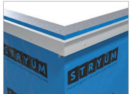
Install the horizontal trims for the cladding, at the top and bottom of the cladding section, above and below any wall penetrations, and at any slab junctions. When installing down to an adjacent flat surface such as a garden bed or pathway, a minimum of 150mm from the ground is recommended to prevent rain splash back dirtying the façade.
