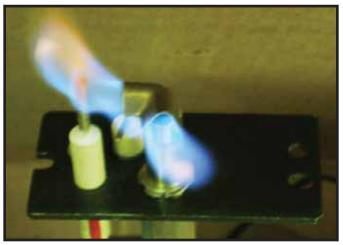
Figure 3.1 IPI Pilot Flame Patterns
