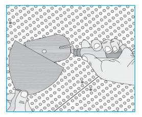
**FIGURE 13 Filling of Screw Heads** (if no Caps used)
