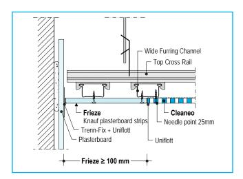
**FIGURE 16 Connection to Wall**
