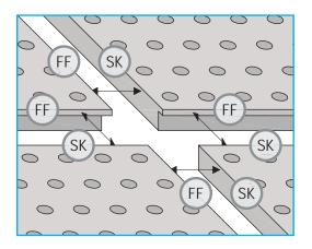
**FIGURE 4 FF Edges Alignment**
