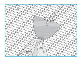
FIGURE 10 'Chipping' Off Excess Filler
