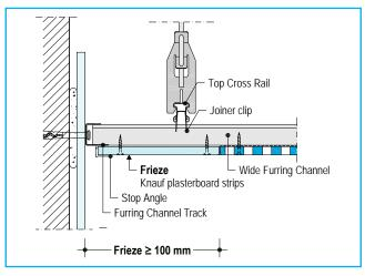
FIGURE 17 Connection to Wall with Exposed Joint
