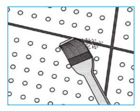
**FIGURE 8 Cleaning of Joints**
