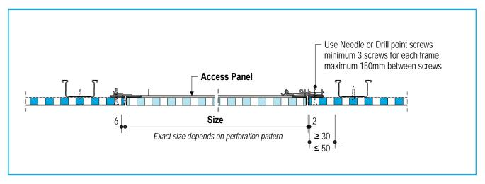
FIGURE 21 Access Panel (with Seal)
