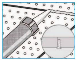
**FIGURE 9 Joint Filling (with Uniflott)**
