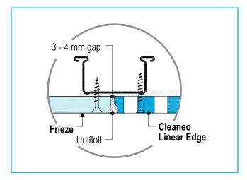
FIGURE 18 Connection to Frieze with Cleaneo Linear Edge
