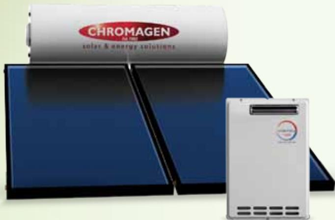
Chromagen's RoofLine solar hot water heaters are traditional close-coupled thermosiphon systems, combining roof mounted solar collectors and storage tanks, which are ideal for applications that are short of available ground space. RoofLine systems are highly efficient and use natural thermal convection to circulate hot water from the collectors to the tank without the need for electric pumps.
