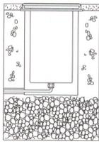
**Note:** STY219RD & STY219SQ Must be mounted in a well drained area. With 20cm of grave.
