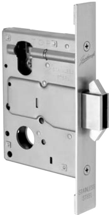
This series is available in a range of functions to suit sliding door applications. Locks are deadlocked by a cylinder and/or turnbutton. The deadbolt has claws fitted to the bolt which protrude or retract behind the strike.
