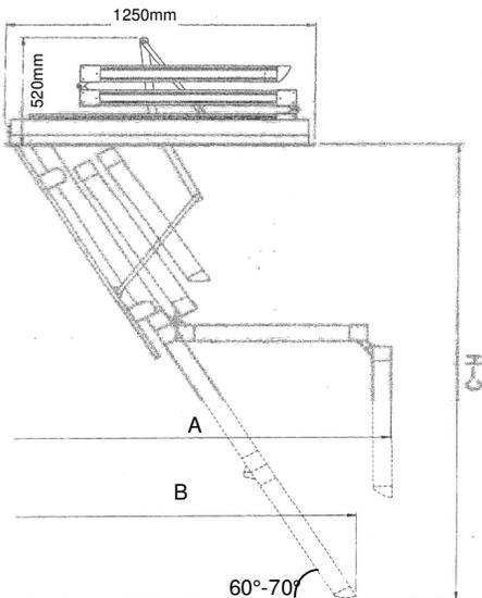
Clearance "A" can be reduced by using a 4-Section ladder.
