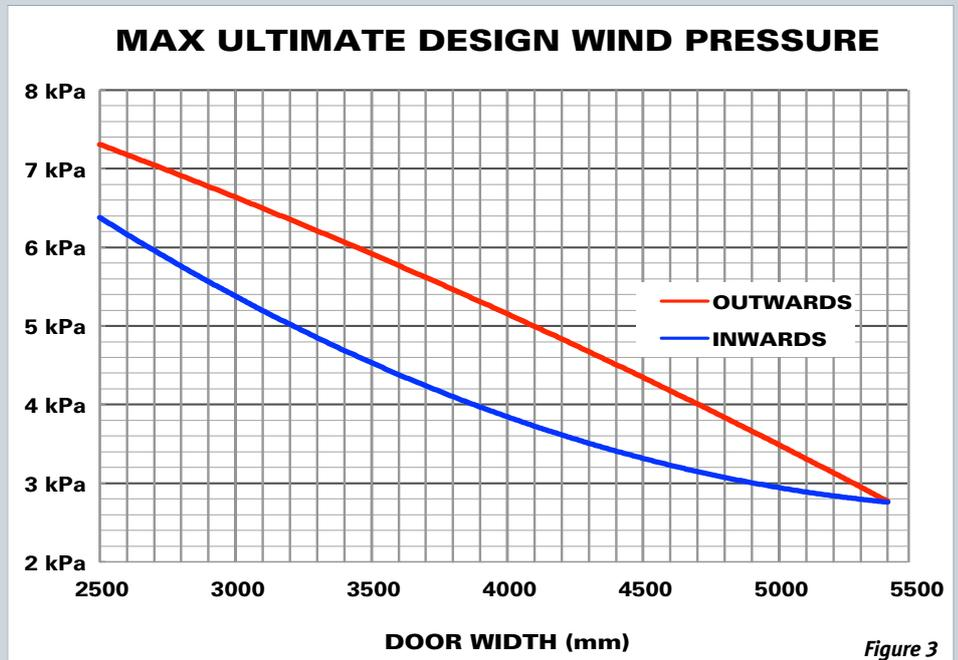
Alternatively, interpolate between lines of Table 2 to find maximum ultimate design wind pressures and maximum abutment forces of other sizes and General Purpose doors. Table 2 gives the forces and ratings of the upper size of the widths from the Taurean Door Systems price list. **Note: Ultimate Wind Pressures in Table 2 may be higher than Wind Classification Pressures available in Table 1 for a particular width.**
