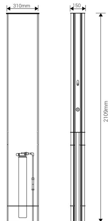
Front & side view with filter detail
