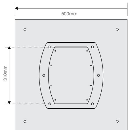
Plan view showing portable base plate
