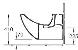
\*Hot/Cold Water Entry points need to be 40mm left & right of centre & 90mm from finished floor
