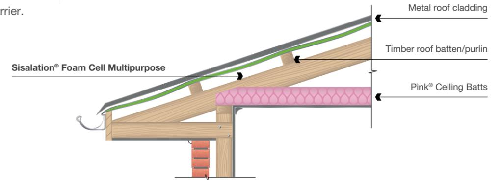
\*Suitability of product for colder climates such as climate zone 6 needs to be confirmed with the building designer. Where Sisalation® Foam Cell Multipurpose metal roof sarking is used, adequate roof ventilation must be provided to minimise condensation occurring within the roof space, refer to state based variations in the NCC for any specific regional requirements.
