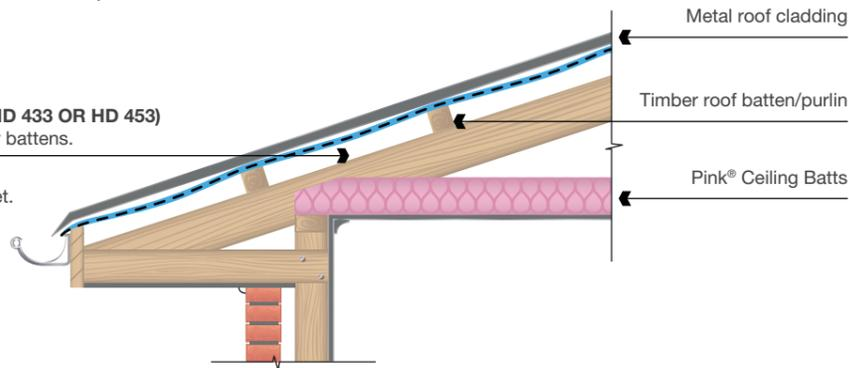
\*Suitability of product for colder climates such as climate zone 6 needs to be confirmed with the building designer. Where Sisalation® Metal Roof sarking is used, adequate roof ventilation must be provided to minimise condensation occurring within the roof space, refer to state based variations in the NCC for any specific regional requirements.
