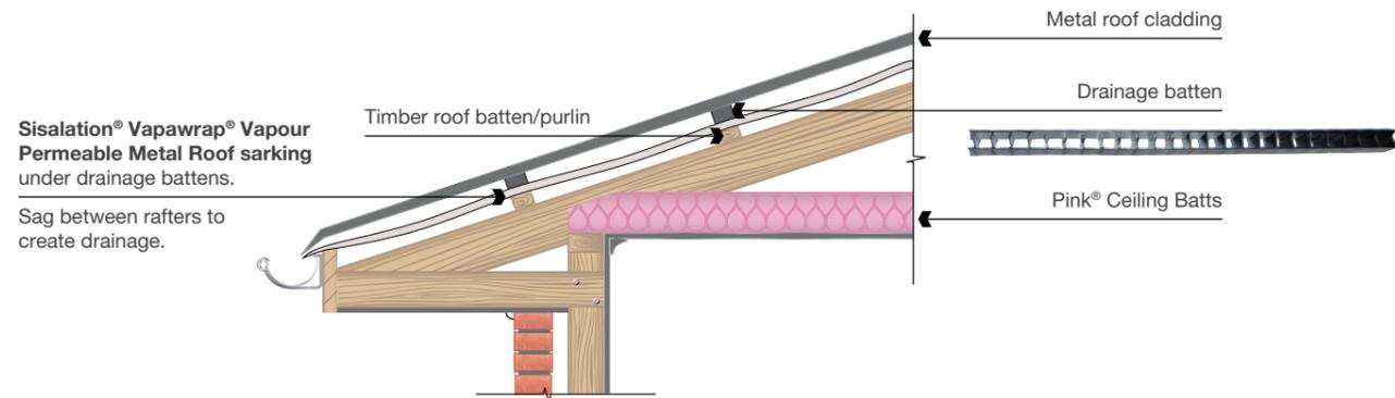
Sisalation® Vapawrap® Vapour Permeable Metal Roof sarking combined with the drainage batten solution provides an effective approach to managing condensation in the roof space by permitting moisture to pass through the fabric as vapour and escape through the ventilated roof cavity. This solution works effectively with higher R-value (>R4.1) ceiling insulation to achieve the overall thermal and acoustic ceiling performance solution.
