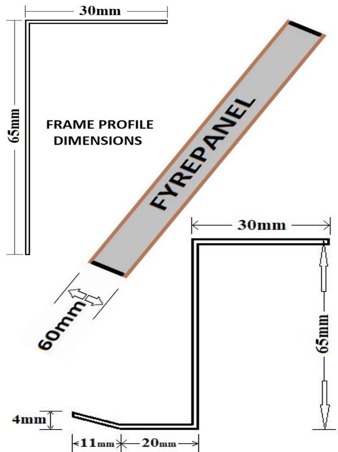
4. Remove panel from frame and install frame into opening using predrilled holes and 10g steel screws. NB: Ensure the frame is temporarily packed out before tightening screws to prevent the frame from distorting. The hatch/panel bolts will not line up with the nuts if distortion occurs. Ensure to remove temporary packers.
