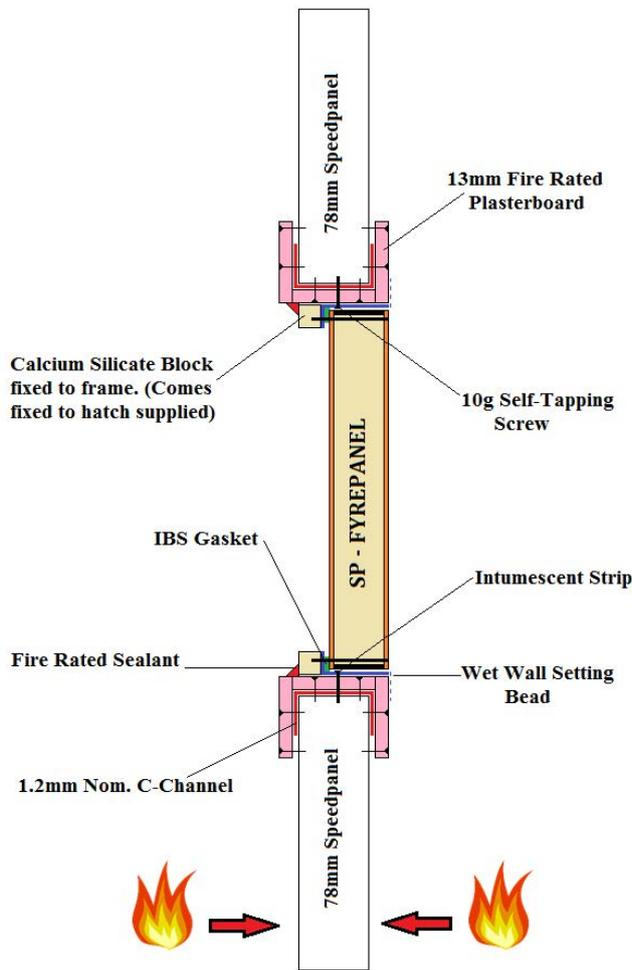
1. Mark out and cut opening in Speedpanel wall approximately 30-32mm larger than hatch frame to allow for trimming of opening.
