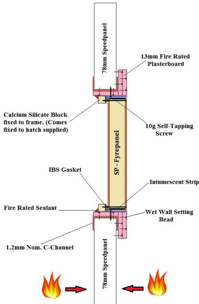
1. Mark out and cut opening in Speedpanel wall approximately 30-32mm larger than hatch frame to allow for trimming of opening.
