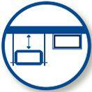
**Space saving** – typically saves up to 150–200 mm in a single dimension, since the space required to manually install a separate layer of insulation around the ductwork is eliminated – this allows ductwork to be installed flush to ceilings, walls and floors, as well as to surfaces within confined enclosures.
