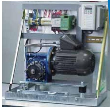
MSL Motor Drive System - internal view
