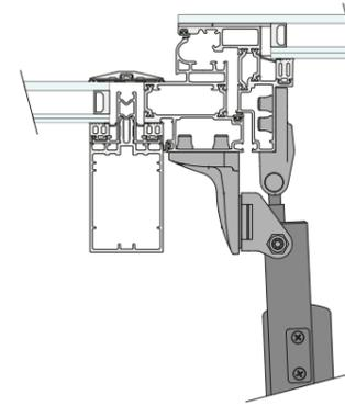
Roof windows, outward opening, side installation
