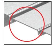
For a weather-tight seal in express jointed facade systems, the central portion of the fixing face is recessed to allow for a self-adhesive foam backing strip.
