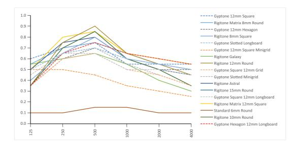
All boards in the Rigitone and Gyptone ranges are supplied with acoustic fabric backing as standard and were tested as supplied, resulting in far better acoustic performance results than Standard 6mm Round, which was tested as supplied without acoustic fabric. Standard 6mm Round is an entry level perforated product, often specified for aesthetics over performance. However, installers may use a third party acoustic fabric to provide far higher levels of acoustic performance if required.
